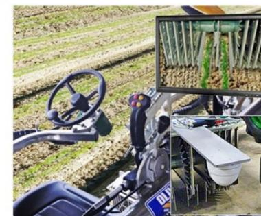
**SISTEMA DI GUIDA MANUALE CON TELECAMERA + MONITOR DA 24"**
