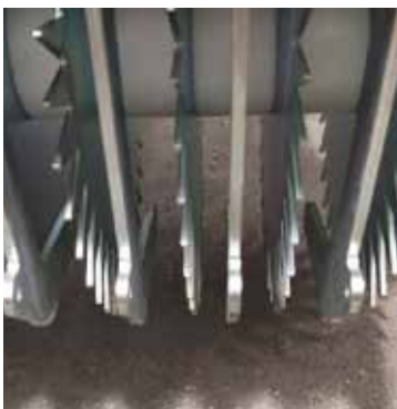
Figure 1 Colibrì, Straight teeth (inter-row spacing 4.5–5 cm)
