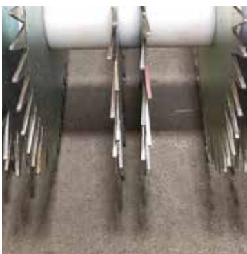
Figure 2 Colibrì, Angled teeth (inter-row spacing 6–7 cm)
